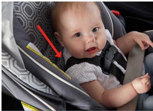
Rear-facing: use the slot at or below the level of the child's shoulders
