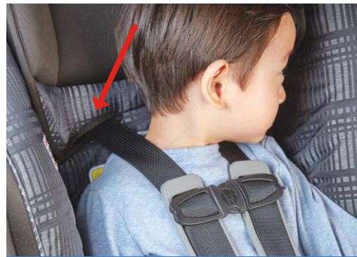
Forward-facing: use the slot at or above the level of the child's shoulders
