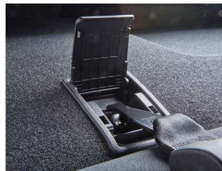
Tether is attached to an anchor behind the rear seat in a sedan
