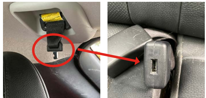
Seat belt stored in roof of vehicle
