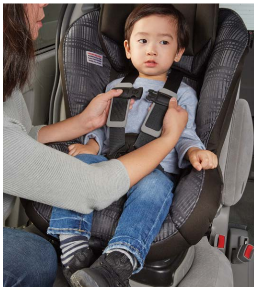
Chest clip is secured at child's armpit level
