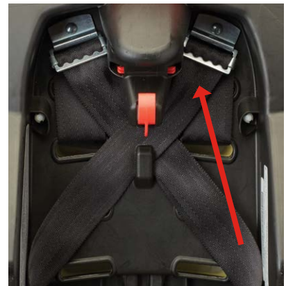
Harness at the back used to loosen and tighten
