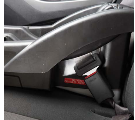
The buckle is twisted enough to bring the latch plate out of the belt path of this base
