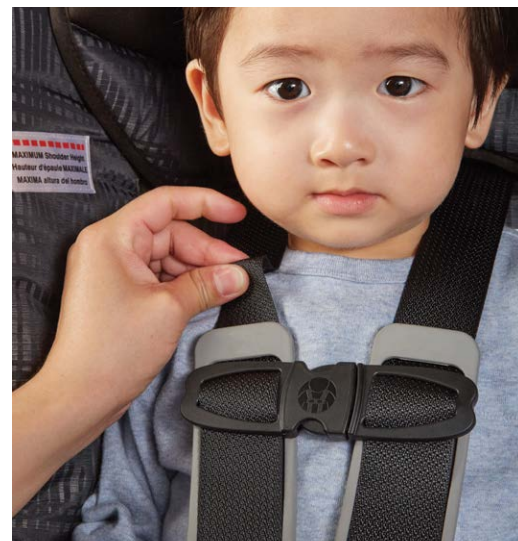
If a fold can be pinched in the harness, it is too loose
