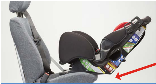
Part of this child car seat hangs over the vehicle seat
