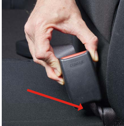
Buckle is twisted to shorten its length
