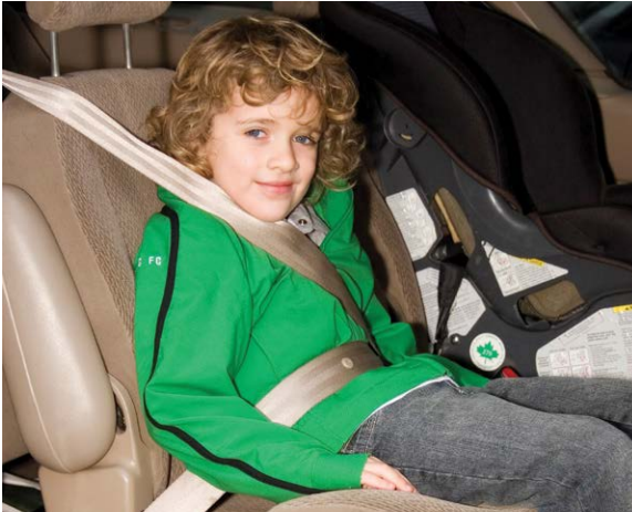
The shoulder belt rubs on the neck, and the lap belt lies across the abdomen incorrectly
