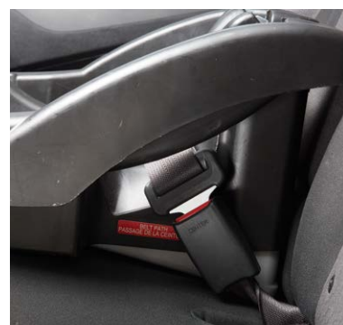
Latchplate and buckle are now clear of belt path
