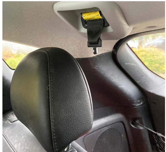
Seat belt stored in roof of vehicle
